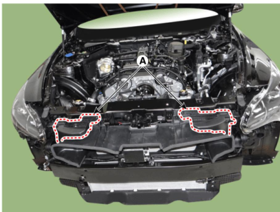
3. Remove the air guard (A) by loosening the bolts after separating the wiring fixing clip.
